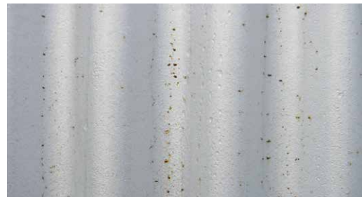
Moderate swarf staining on ZINCALUME Plus.
