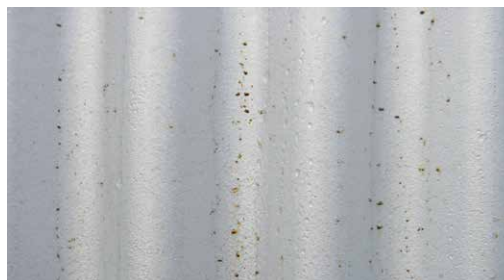
Moderate swarf staining on ZINCALUME Plus.
